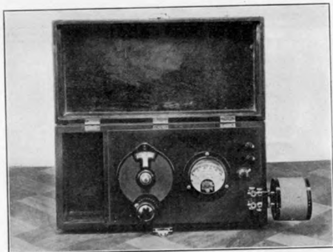
Fig. 1. The simpler the design, the more accurate the wavemeter
