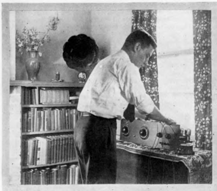
Fig. 1. M. B. Sleeper, checking the voltage on the tubes with a Jewell table-meter, before installing the set in the cabinet—Photographed in a corner of the library in the New York Laboratory
